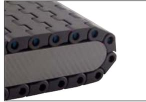
The 2120 series belt with 1/2" pitch and concave bottom is very well suited for nose bar transfers. The small pitch and the concave bottom reduce the polygon effect to an absolute minimum.
