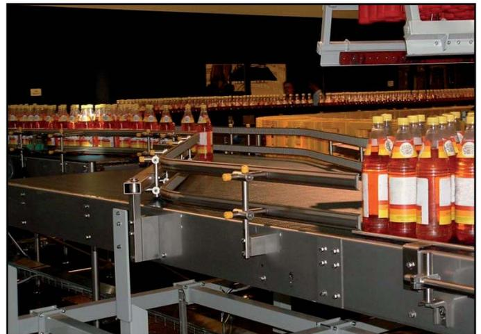
There's also a completely flexible execution that allows a flexible radius or a twisted roller guide.
