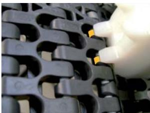
Sprockets engage on the curved end of the hinges. The teeth of the sprocket must push the highlighted surface of the hinges. That is important for the installation of sprockets.
