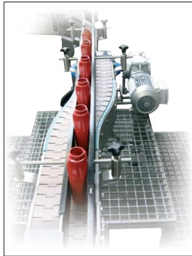
Instead of the products shifting sideways onto the next chain, the chain is shifting from underneath the products. The side guide remains straight and the pressure on the products is less. This transfer system always requires a side flexing chain.
