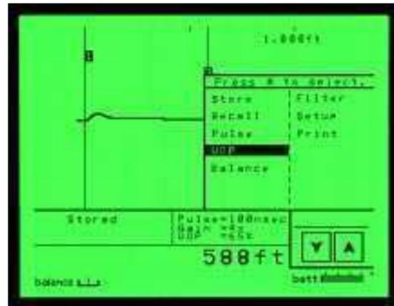
A balanced test port minimizes the blind spot associated with the TDR test pulse and matches the instrument to the cable under test. This helps locate faults close to the instrument.
