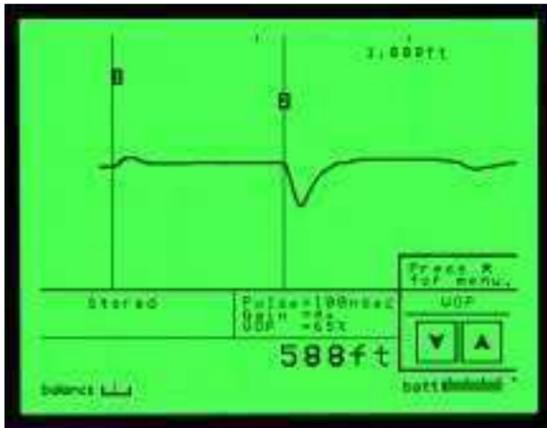
Selected functions and operations are controlled by the keypad, such as waveform position, horizontal zoom, vertical gain, cursors, range, contrast, and backlight. A popup menu is easily accessible for additional functions. Riser-Bond Instruments' unique popup menu system allows the operator to select and use a function while the waveform is active.
